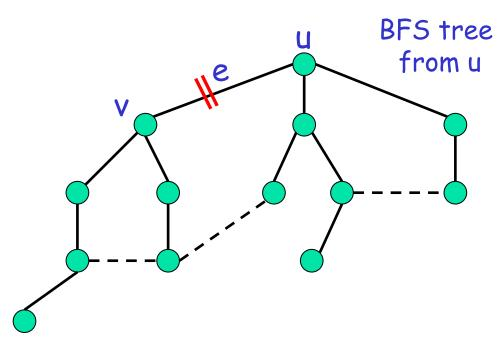
Let G be a network with diameter d, and let e=(u,v) be a non-cut edge. Then in G-e, every node w increases its distance from u by at most 2d
