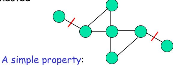
Any graph has at most n-1 cut edges (indeed, if we take any spanning tree T of G, all the non-tree edges cannot be bridges, and T has exactly n-1 edges (not all of them are bridges, clearly))
